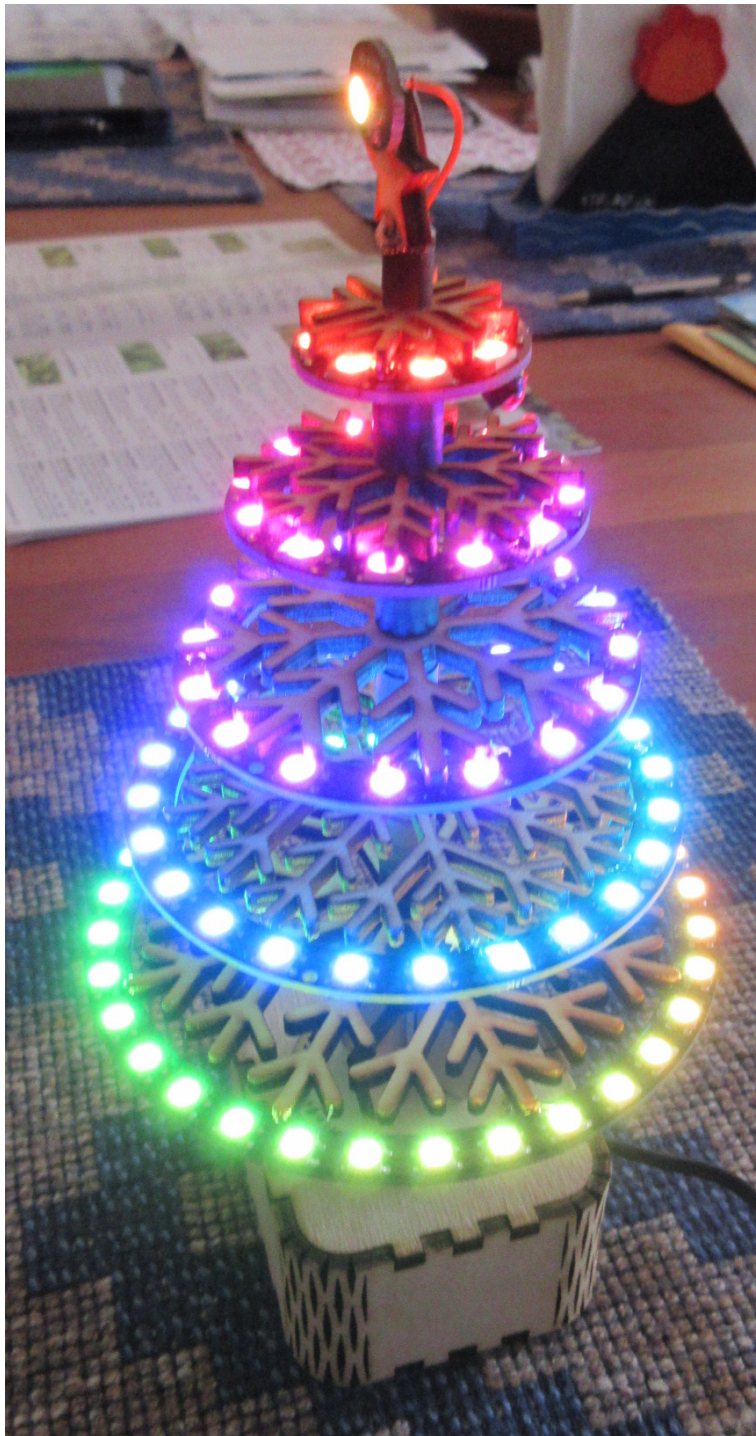
Figure Eleven Finished and Operational NeoPixel LED Tree
